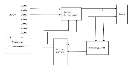
Fig: Block Diagram of tap changer Transformer
