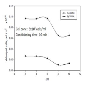
Fig. 7. Effect of pH on Adsorption of P. polymyxa onto single minerals
