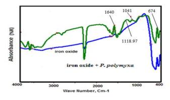
**Fig. 10**. FTIR spectra of hematite after treatment with P. polymyxa
