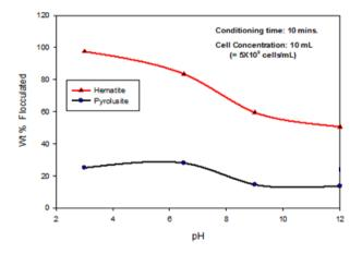
**Fig. 11.** Flocculation power of single minerals using 10 ml (5x109 cells/ml) P. polymyxa at different pH values
