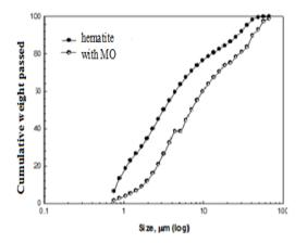
Fig. 3. Effect of P. polymyxa on Size Distribution of Hematite
