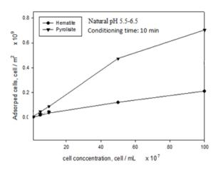
**Fig. 8.** Adsorption Isotherm of P. polymyxa onto minerals' surfaces
