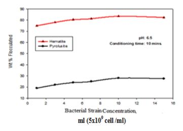
**Fig. 12**. Flocculation of Single Minerals as a Function of Concentration of P. polymyxa at pH6.5
