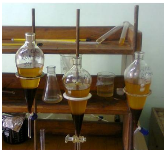
Fig 2.1: Separation of Glycerol from Linseed methyl ester
