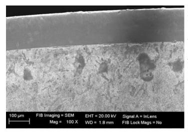
Fig-6 SEM image of coated plate
