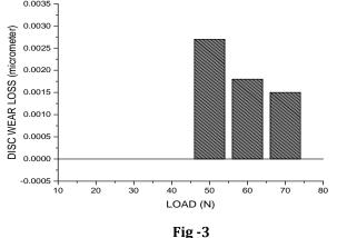
On rubbing between pin and disc, friction heat generated due to which there is a loss of both material i.e. wear loss.
