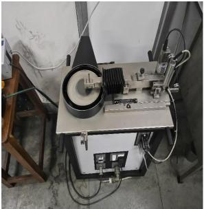
Fig -1: Pin-on-disk tribometer
