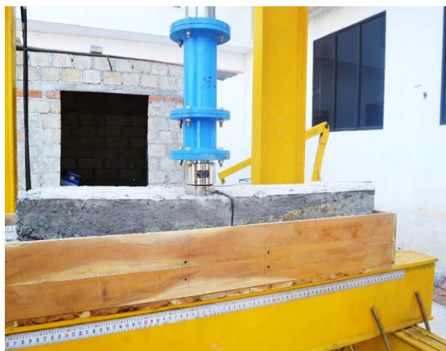
Fig 11: Testing of slab specimens
