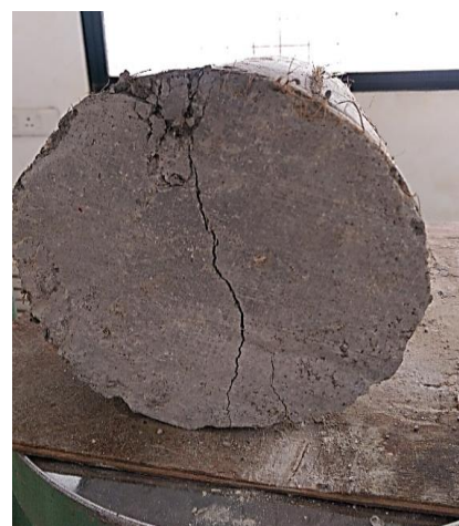
Fig 8: Splitting tensile strength test of specimen with fibre.
