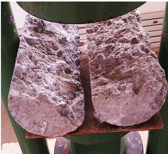
Fig 9: Splitting tensile strength test of specimen without fibre.
