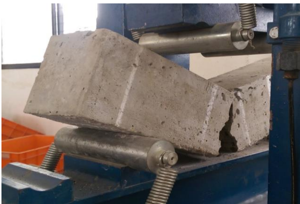
Fig 6: Flexural test specimen without fibre
