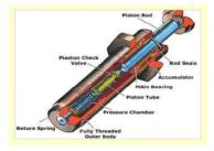
(1.1) MAIN COMPONENT OF SHOCK ABSORBERS ARE: (a) PISTON ROD,(b) MAIN BEARING,(c) PISTON RINGS,(d) PRESSURE CHAMBER, (e) OUTER BODY
