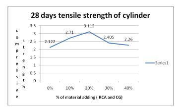
The value obtained for 20% and 30% for the 7 days curing addition of recycled coarse aggregate and water cement ratio 0.5 yielded highest results for tensile strength and 10% and 20% for 28 days curing. However, the tensile strength decreased on the increase in RCA and CG addition. Therefore there is an optimum value of RCA ,CG to cement ratio, beyond which the tensile strength decreases. Hence 0.5 was taken as the optimum water cement ratio and optimum RCA and CG content was taken as10% & 20%.
