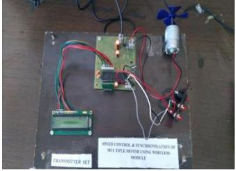
Fig 6. Hardware model of Transmitter
