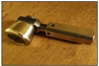
Fig -2: Single Roller Burnishing Tool
