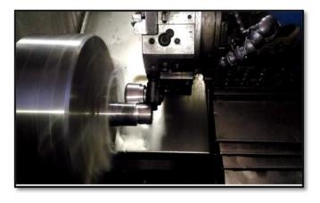
**Fig -3**: Experimental setup of roller burnishing operation on CNC lathe.
