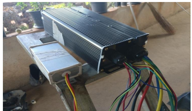
Figure 3. VOLTAGE REGULATOR (R) AND MOTOR CONTROLLER (L)
