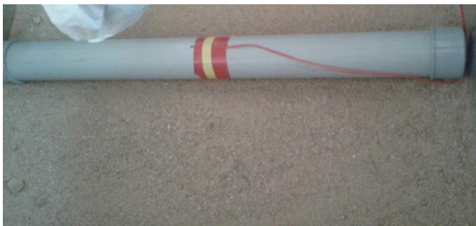
Fig -1: strain gauge mounted on pipe
