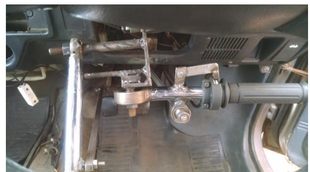
Fig -18: Complete Assembled Hand Controls to Vehicle
