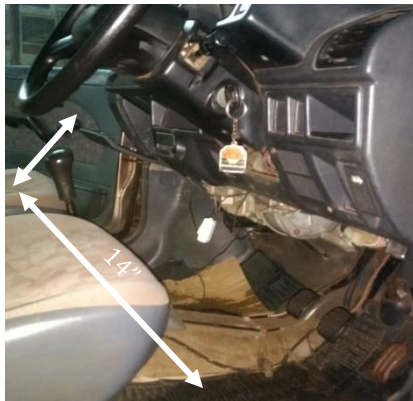
Fig -12: Distance between Pedals & Driver underside the Steering Column
