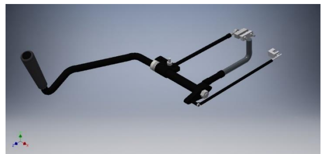
Fig -9: CAD Model of Push - Pull Mechanism
