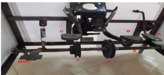
MAC: MAC pedal, C: Clutch pedal, P: Pulley, B: Brake pedal, A : Accelerator pedal, S: Shaft
