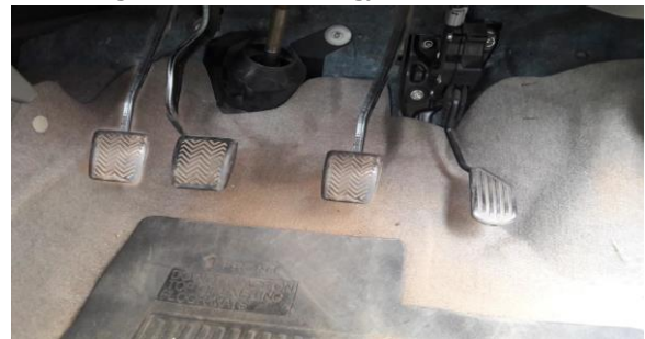
Fig 4: Arrangement of MAC pedal in Tata safari
