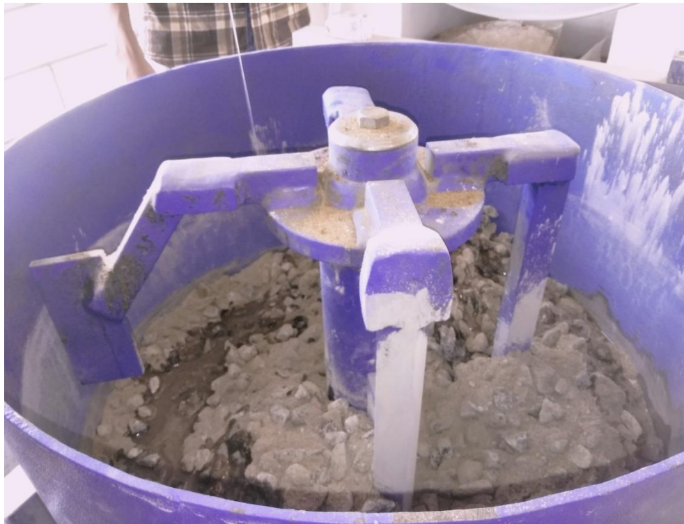
Fig. 2 Pan mixer user for mixing geopolymer concrete
