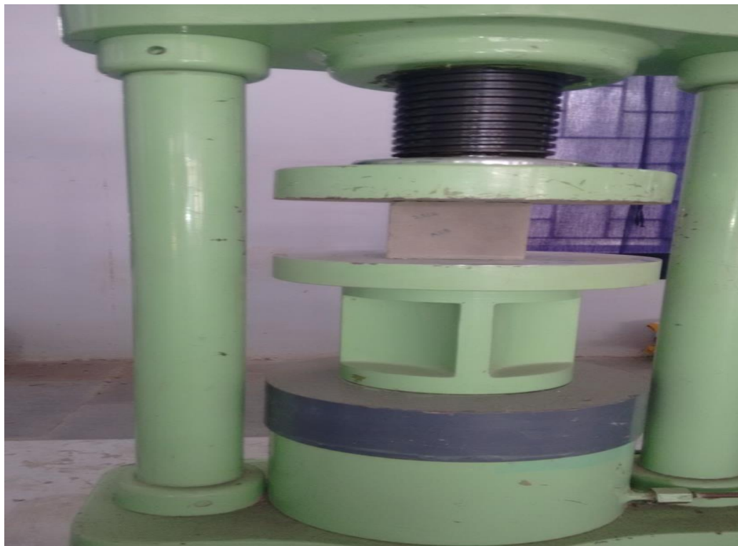
Fig. 4 Compressive strength testing of geopolymer concrete
