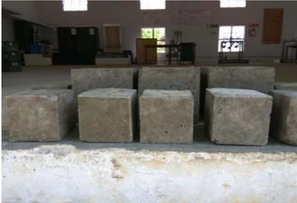
Fig. 3 100mm geopolymer cubes after demoulding
