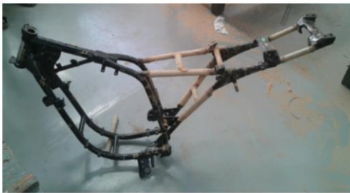
Figure 13:-Chassis frame with use of bamboo and steel
