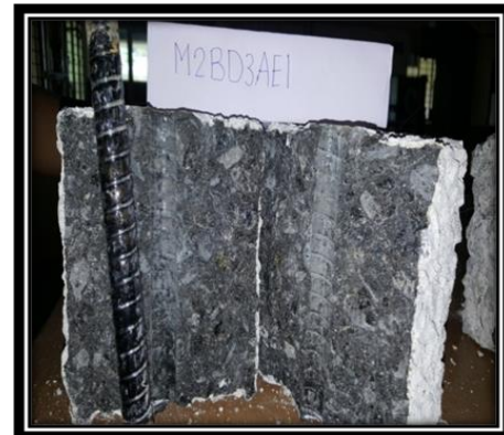
Fig -4: Concrete splitting mode of failure
