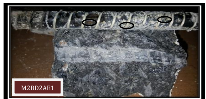
Fig -6: Brownish traces observed in the bar
