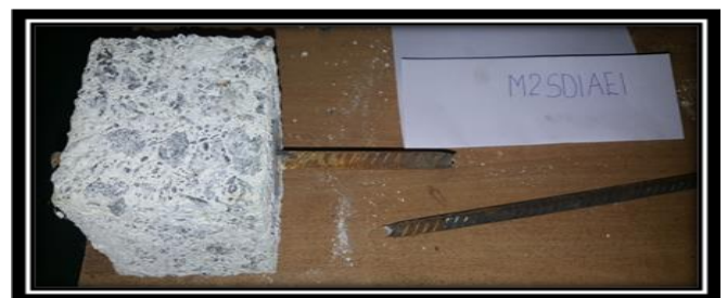
Fig -5: Steel rupture mode of failure
