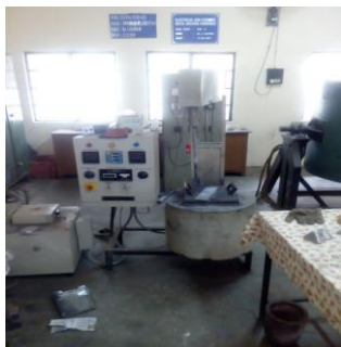
Figure-1: Stir Casting Equipment
