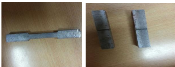
Figure -2: (a)Tensile specimen(b)impact specimen
