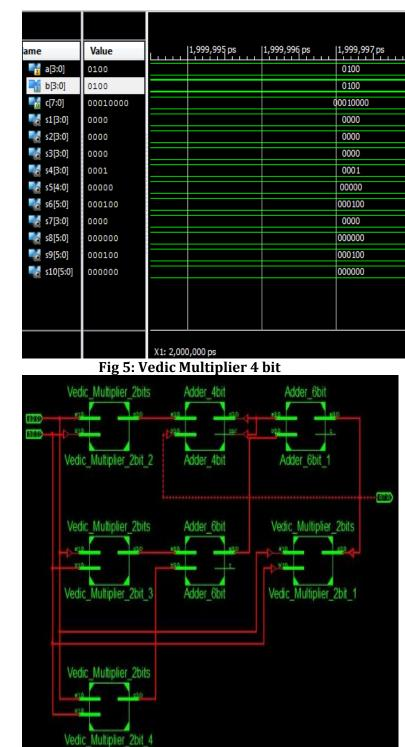
Fig 5: RTL Schematic of 4 Bit VEDIC **Multiplier**
