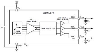
Fig -5: Functional block diagram of ADXL377 [3]
