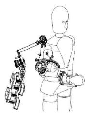
Fig. 6. CAD model of L-EXOS
