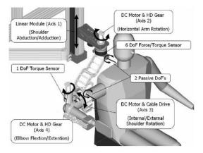
Fig. 7. The Mechanical Design of Robot
