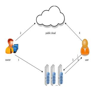
1. Owner registers with the secure server and obtains credentials to upload data to cloud.
