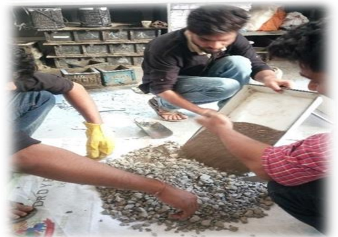
Figure-2: Mixing of dry aggregate
