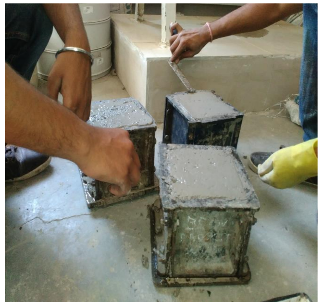
Figure -3: Casting of GPC cube
