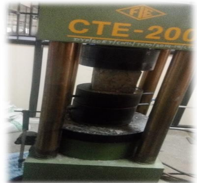
Figure -5: Compression test on concrete cube
