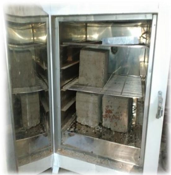
Figure- 4: Oven Curing for GPC cube
