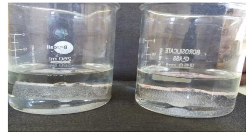
Fig 3. Corrosion test samples in solution
