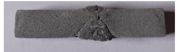
Fig 4. Specimen 1: After corrosion
