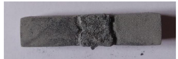
Fig 5. Specimen 2: After corrosion
