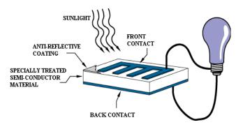
Fig.2 Working of Solar Panel
