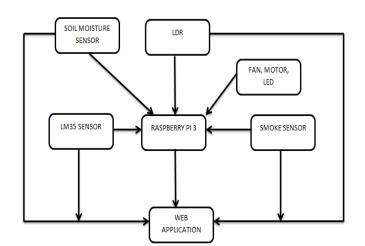
Fig -1: Block Diagram of Smart Agriculture Management System
