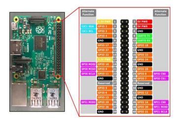
Fig -4: Pin Diagram for Raspberry Pi model 3
