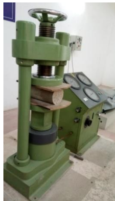
Fig-13: Split tensile strength testing machine
