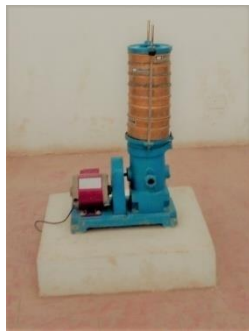
Fig-4: Sieve analysis on fine aggregate
