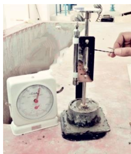
Fig-6: Consistency test
