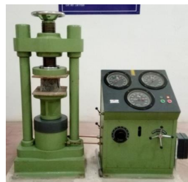
Fig-12: Compression testing machine
