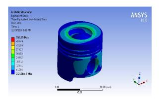
Case 6: For pressure = 15 N/mm<sup>2</sup> (For Cast Iron)
