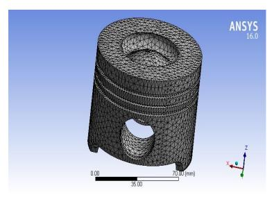
Fig 3: Meshing of Piston Model
