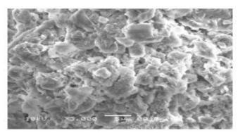
Fig-3: SEM image of soil mixed with 100% textile effluent
