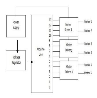
Fig -2: Block diagram of electrical assembly
