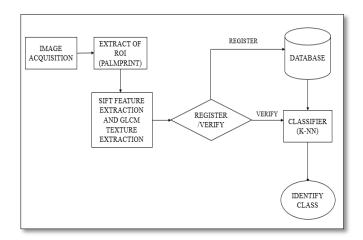
In the following module, features are extracted using local and texture feature. Then, these features are matched with the feature enrolled in the database and palm print is identified using nearest neighbor classifier.
