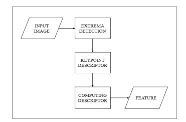
Figure 2: Block Diagram of SIFT
