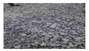
Almost all materials which are used in the construction industry were entirely natural and all waste from demolished buildings was disposed of in landfills and partially in unauthorized places. The utilization of the recycled aggregates created from processing C&DW in new construction has become more important over the last two decades.
