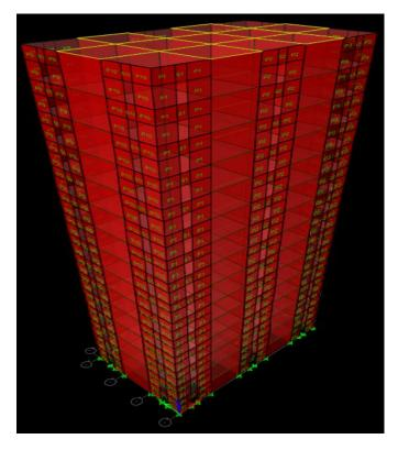
Fig 1.2:Coupled Shear wall 3d view
