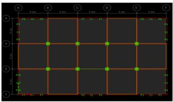
Fig 1.1:Coupled Shear wall plan layout
