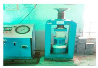
Fig.3: - Compression testing of cubes
