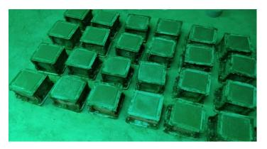
Fig. 2: - Concrete Cubes ready for curing
