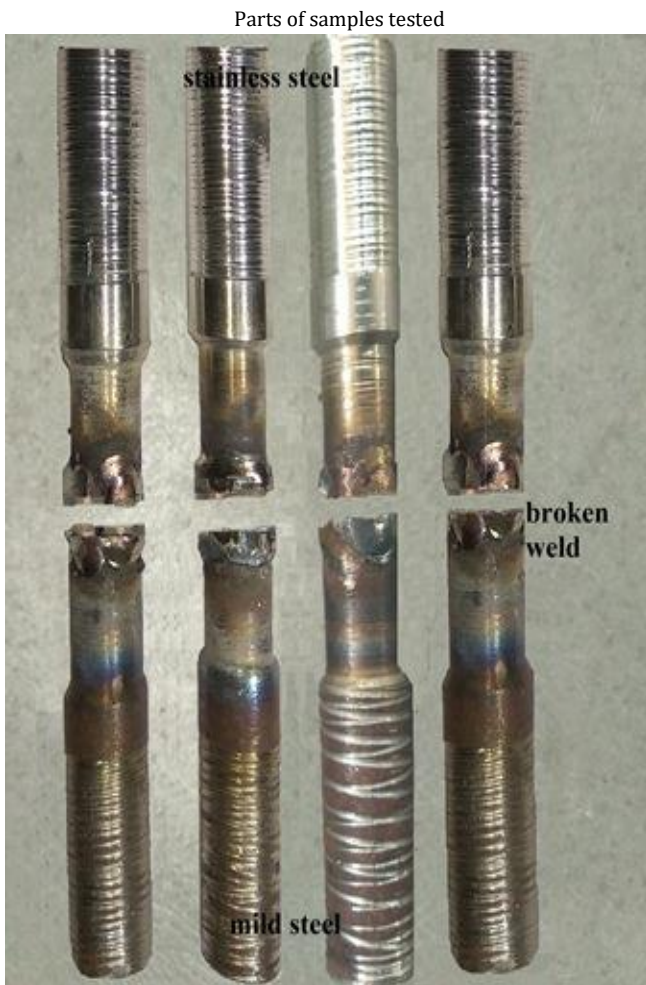
Fig-6: Tested Welds in UTM
