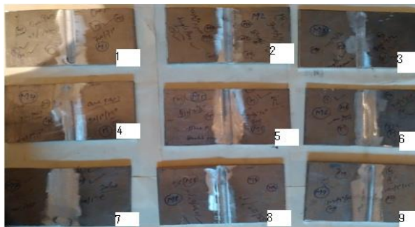
Fig. 5 Welded Parts by square tool for multipass
