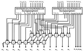
Fig. 3. CSA based 8×8 signed row bypassing multiplier
