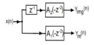
Figure 1. Realization of Complex half-band filter using All pass filter.
