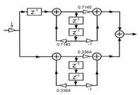
Figure 4. Realization of Direct form II Hilbert Transformer
