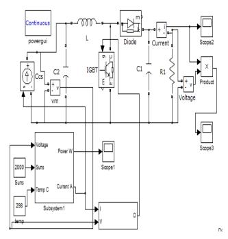
**Figure.6.** the solar modeled of PV system with inverter
