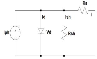
Figure.2. Solar cell equivalent circuit
