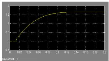
Figure.8. Current graph without any controller
