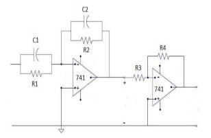
Fig-2: Circuit diagram of lead compensator
