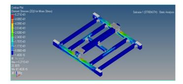
Fig. 6 Top Frame Stress Plot
