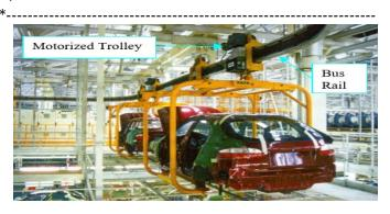
Fig. 1 Actual Setup of Conveyor System
