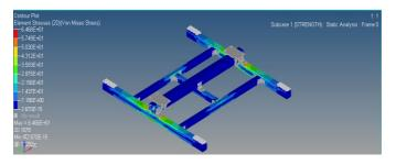
Fig. 7 Optimized Top Frame Stress Plot
