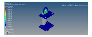
Fig. 4 Optimized Trolley Stress Plot
