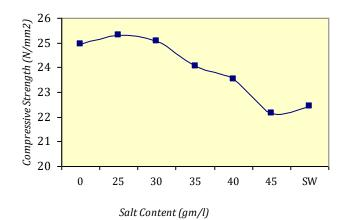
**Fig - 1**: Showing Average Compressive Strength of cubes at 3 Days Curing.
