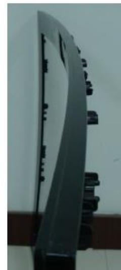
Fig -6: Warpage on the front surface of LCD TV shell [1]
