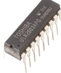
Fig -3: IC ULN2803 APG
