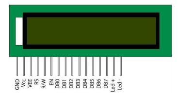
Fig: 4. Pin Configuration of LCD
