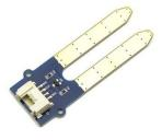
Fig: 3. Moisture sensor (Model: SEN92355P
