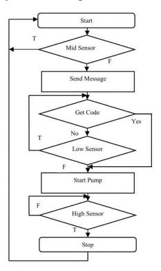
Fig: 1. Flow diagram of automated irrigation system
