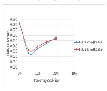
**Chart-4:** Comparison of failure strain of clay stabilized with various Percentages of tire scrap
