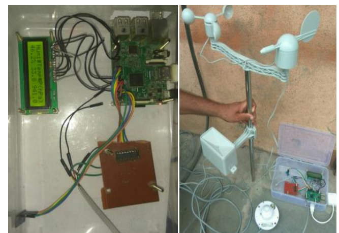
(a) Raspberry Pi with LCD Display and ADC (b) Sensor Unit
