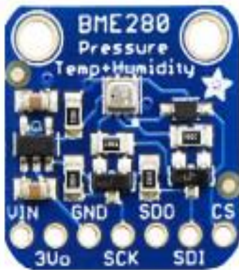
Fig. 6. BME 280 (air temperature, humidity, Atmospheric pressure sensor)
