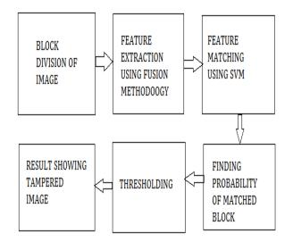
FIG-2: Block Diagram Of Proposed Method
