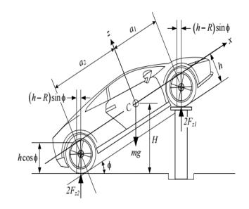
FIG 2.2 Measuring the forces under the wheels to find the height of mass center
