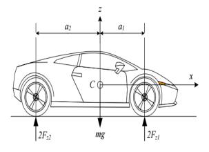
FIG 2.1 A parked car on level pavement
