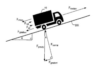
FIG 3.1 FBD of moving vehicle
