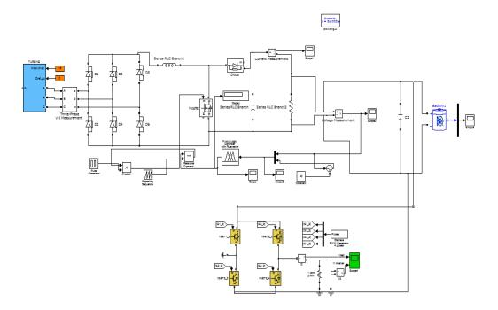
Fig. 6..MATLAB/SIMULINK diagram of the proposed fuzzy based WECS.
