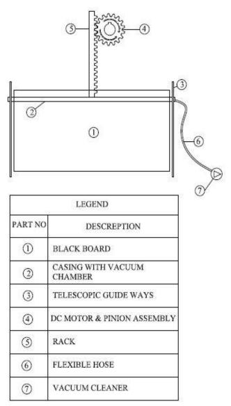
Fig 4: Assembly of components
