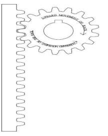
Figure 1: Rack and pinion arrangement
