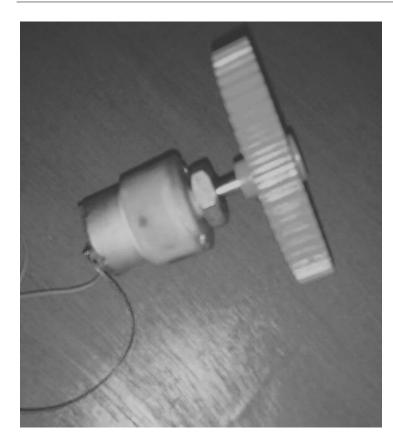
Fig 3: DC motor and pinion assembly
