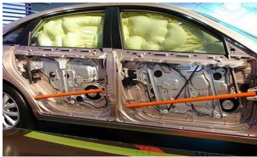
Fig 3.1: Hyundai Azera showing the side impact beams and the side impact airbags deployed.
